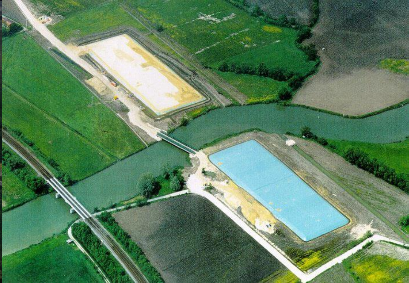
Boutonne River crossing (One zone is simply under vacuum, the other one is already filled)
