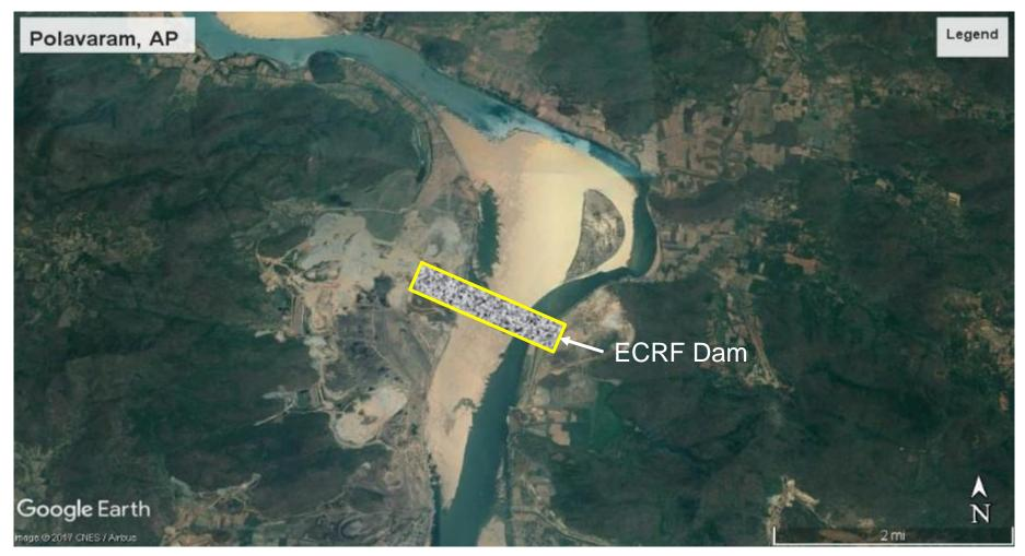
VC works below the Earth cum Rockfill (ECRF) Dam to mitigate liquefaction & enhancing overall stability of dam
