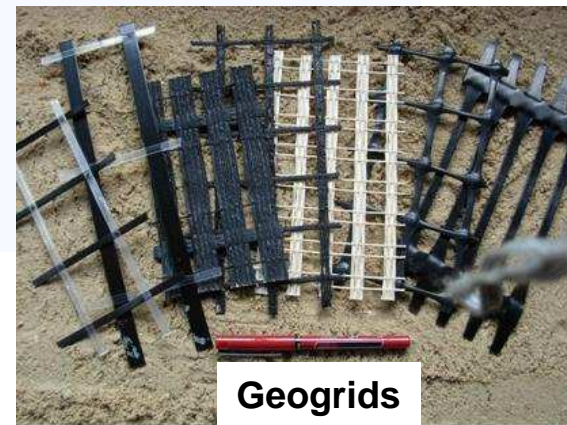
High-tenacity polyester yarns protected by polyethylene sheath
