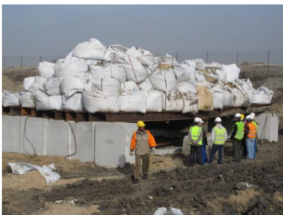
Photo 3 : Excessive vertical displacement of the improved ground during plate load test
