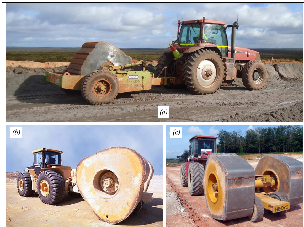
Photo 1: Rolling dynamic compaction modules: (a) 4-sided (Broons), (b) 3-sided (Landpac), (c) 5-sided (Infratech).
