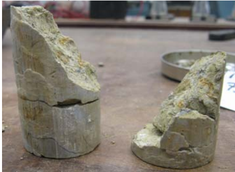
c, 32_TRI(75)_N. Wavy failure plane
