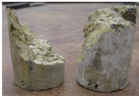
d, 32_TRI(50)_L Curving failure plane
