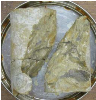
a, 8_TRI(25)_N Slickensides on failure surface
