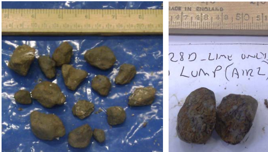
Figure 3: a (left) 'Stiff' nodules recovered from 32_CBR_L. b (right) A nodule split in half.
