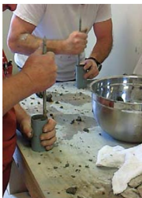
Photo 3.1 Filling condition to molds
