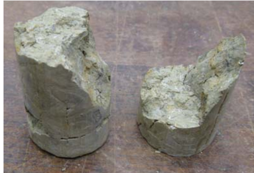
b, 32_TRI(25)_L Abrupt change in failure plane
