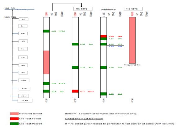
Figure 7: Test Results of the DSM Column showing the inconsistence of the original method
