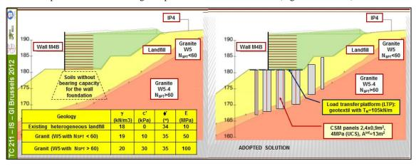
Figure 22: Cross section geological conditions and adopted solution.
