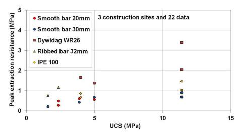
Figure 16: Peak pull-out resistance in function of the UCS of cored DSM material
