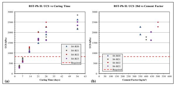
Figure 5: BST - Phase II results (a) UCS vs Curing time; (b) 28 days UCS vs Binder Factor
