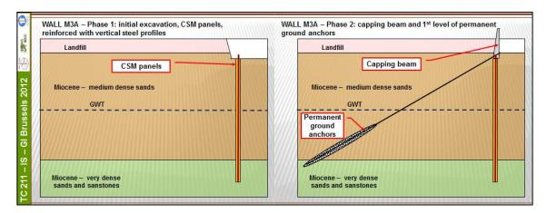
Figure 11: Construction phases 1 and 2.
