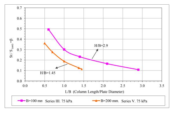
Figure 4:  $\beta$  – L/B relation for series III and V for 75 kPa loading
