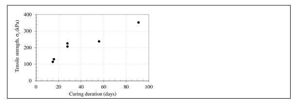
Figure 6: Evolution of tensile strength with curing duration
