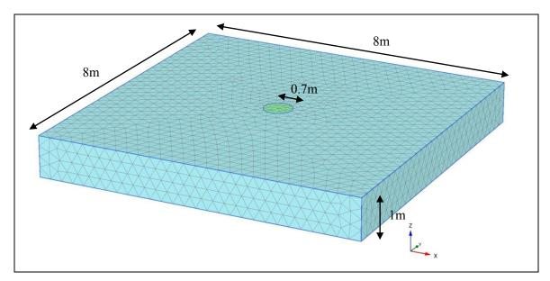
Figure 1: Volume pile model without interface elements – medium mesh density
