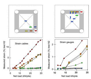
Figure 8: Measured strains occur mainly in the tensile strips that lie on the GR strip between adjacent piles, in accordance with the calculation models (see Figure 1).,
