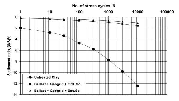
Figure 8: Number of stress cycles versus settlement ratio for different model tests at constant stress
