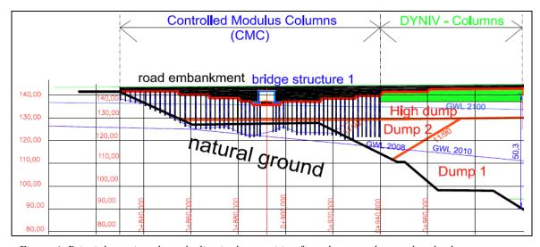
Figure 4: Principle section along the line in the transition from the natural ground to the dump
