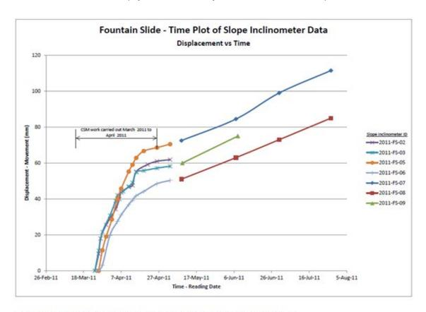
\*Note: Slope Inclinometer 2011-F5-02 to 2011-F5-06 were damaged by site equipment. 2011-F5-07 to 2011-F5-09 were installed as replacements
