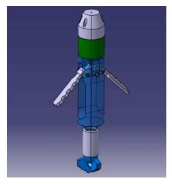
Figure 2: New soil-mixing folding tool FLAPWINGS
