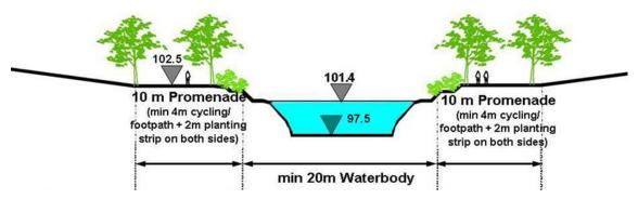
Figure 3: Cross-sectional View of the Punggol Waterway
