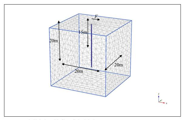
Figure 5: Embedded pile model of laterally loaded pile
