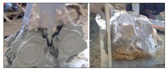
Figure 15: Cutting head used to the execution of the CSM panels (on the left) and example of a rocky block collected during the excavation (on the right).
