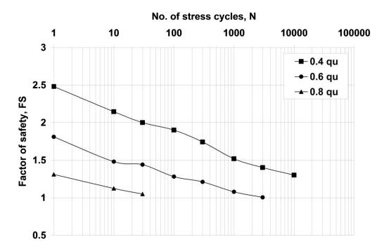
Figure 3: Factor of safety versus number of stress cycles for untreated soil
