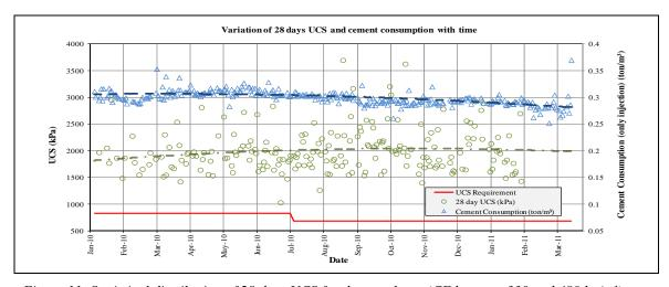
Figure 11: Statistical distribution of 28 days UCS for the peat layer (CF between 330 and 480 kg/m³)
