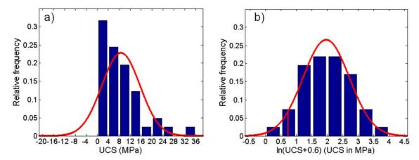
Figure 17: a) Distribution of the UCS values of 41 cores of DSM material from a site in Gent and the corresponding theoretical Gaussian curve. b) Distribution of the logarithm of the UCS values of the same site but increased with  $\beta = 0.6$  and the corresponding Gaussian curve. The vertical red line indicates the 5% lower limit value
