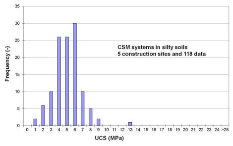
Figure 4: Histogram of the UCS test results for CSM systems in silty soils
