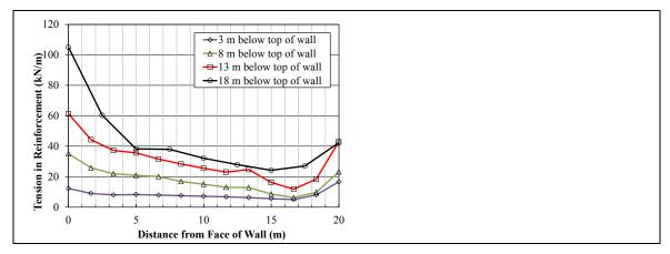
Figure 6: Plot of tension in the MSE reinforcement as a function of the distance from the face of the wall
