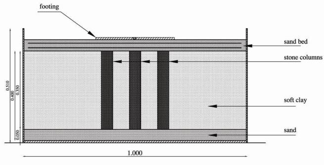
Plate. 1 schematic diagram of the apparatus
