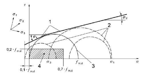
Figure 5: Allowed stresses inside a deep mixing bodey according to [8, Picture 1] © DIN
