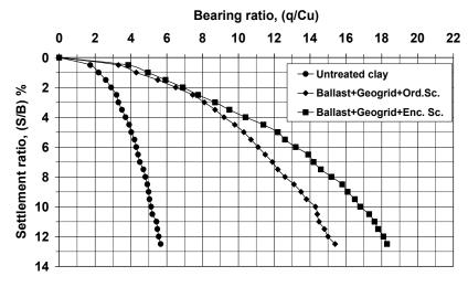
Figure 1: Model test Results- Monotonic loading-
