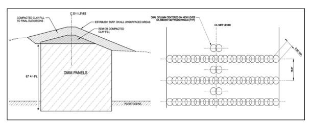
Figure 2: typical design of DMM stabilization at LPV111 (cross section & plan view)
