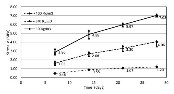
Figure 2: Evolution of unconfined compressive strength of specimens of soil mixing depending on curing time (for different cement contents).
