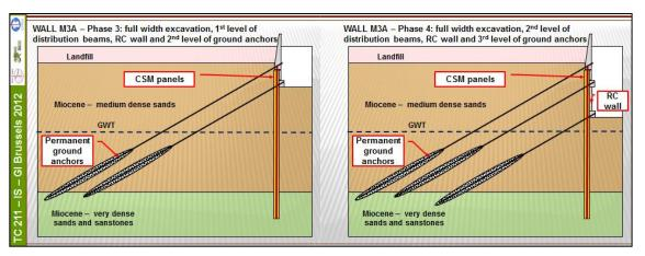
Figure 12: Construction phases 3 and 4.
