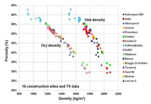
Figure 12: Relationship between dry and wet density and porosity for DSM cores
