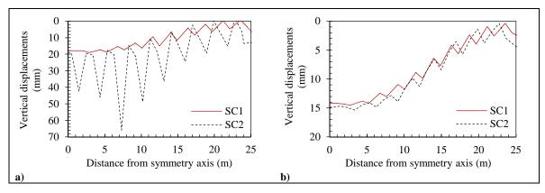
Figure 3: Settlements at the completion of calculation phase #6: a) embankment base, b) at the depth of 10 m
