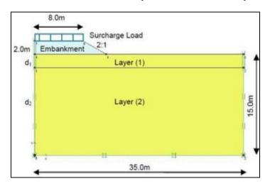
Figure 1: Numerical model (Plaxis-2D-V8) [4]
