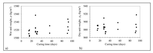
Figure 3: Evolution of (total and dry) density with curing time
