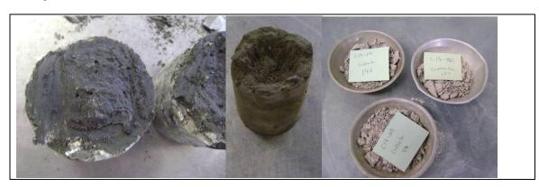
Photo 4: Water content determination of cylindrical specimen preparation after unconfined compression test
