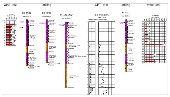
Figure 4: boring, cone penetration test and shear vane test in the detail area bridge west
