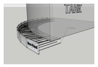
Figure 4: Conceptual view of the MSE Ring Wall
