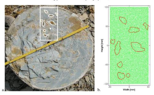
Figure 2: a. Section through a soil mix column; in this section a rectangular sample with dimensions of 120×240 mm is selected; b. Mesh generated for the discontinuous simulations (red lines indicate the soil inclusions)
