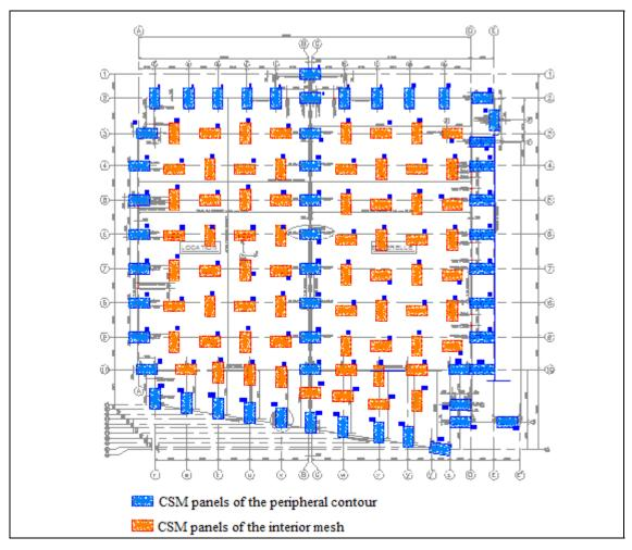
Figure 7: Plan view of CSM panels distribution.
