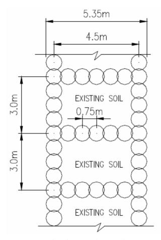
Figure 5: Typical Grid Pattern of Deep Soil Mixing (DSM) Columns.
