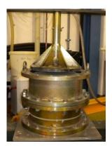
Figure 4: Consolidation of the slurry in a container
