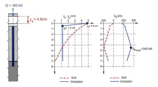
Figure 7: Step 3 of the calculation according to the simplified method - Inclusion diameter 0.34 m, vertical load case q = 200 kPa
