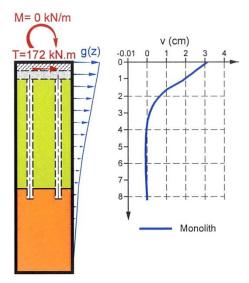
Figure 9: Step 4 of the calculation, according to the simplified method - Monolith cross-section area 2.8  $m^2$ , inclined load case q = 200 kPa,  $\theta = 10^\circ$
