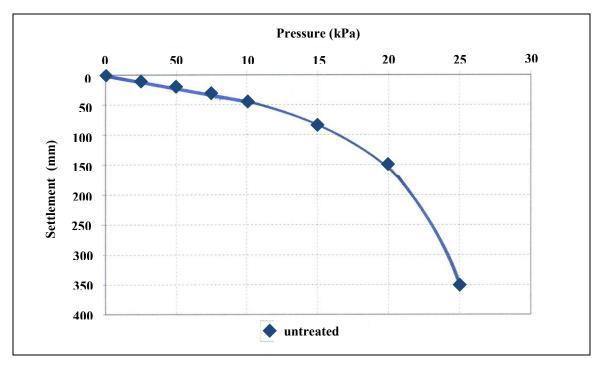
Figure 2: Surface settlement- pressure relationships for untreated soil
