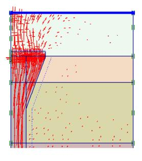
Figure 6. Friction along the pile (maximum 110 kPa)
