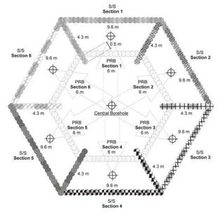
Figure 6: Schematic of the hexagon of inner PRB walls and outer low permeability walls.
