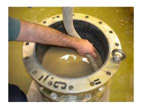
Figure 3: Pouring slurry into the container
