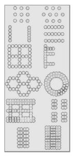
Figure 2: Design of the soil mixing columns [Topolnicki, 2006]
