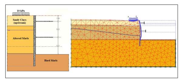
Figure 7: Section A: cross-section (on the left) and analysis model representing the deformation at the maximum excavation depth (on the right).
