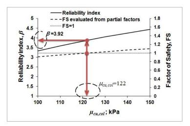
Figure 5: Partial factor design for the design of the embankment, the partial factors for only the important parameters ( $c_{u,col}$ ,  $c_{u,soil}$  and  $\gamma_{emb}$ ) were considered and evaluated from FORM analysis
