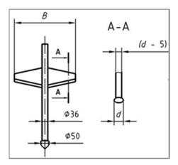
Figure 6: Test probe for column penetration test [DIN EN 14679]
