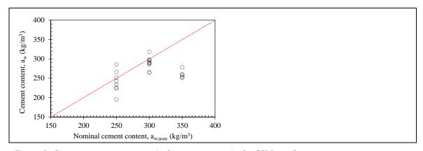
Figure 1: Cement content versus nominal cement content in the CSM panels
