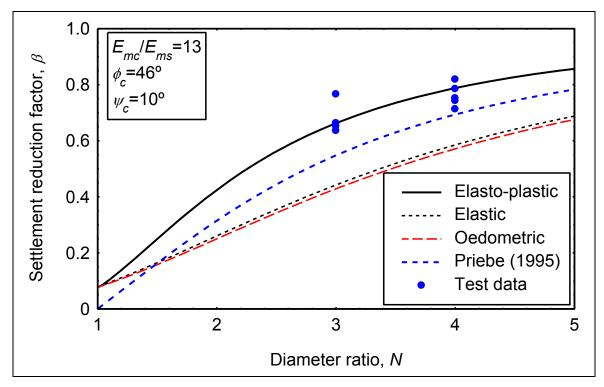
Figure 5: Comparison of the settlement reduction factor.
