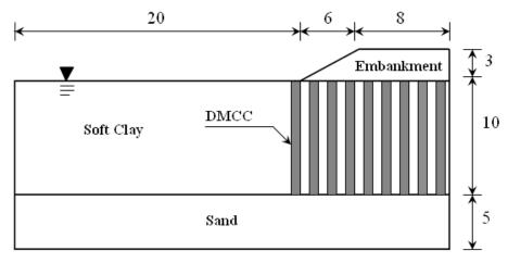
Figure 1: Half section view of embankment on DMC columns (all dimensions in m)
