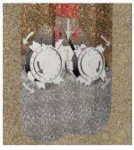
Figure 3: Construction process in Geomix technique with CSM equipment
