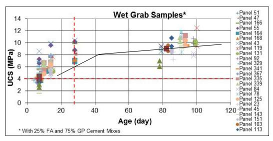
Figure 2: Results obtained from the UCS tests on wet grab samples from production columns
