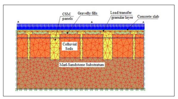
Figure 10: Simplified geometry, finite elements mesh and boundary conditions of the numerical model.
