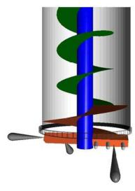
Figure 4: Scheme of the TSM mixing tool (Smet-F&C)
