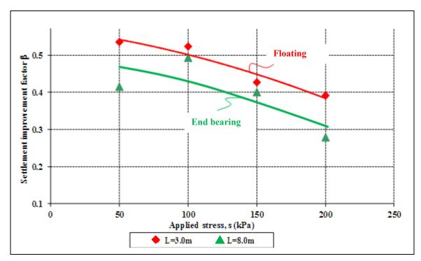
Figure 4: Variation of  $\beta$  ratio with applied pressure
