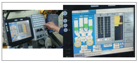
Figure 4: Rig operator's monitor to the control of execution parameters.
