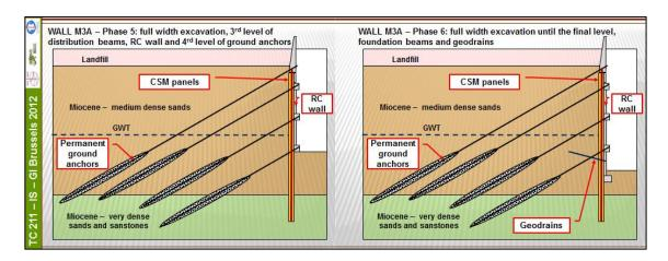
Figure 13: Construction phases 5 and 6.
