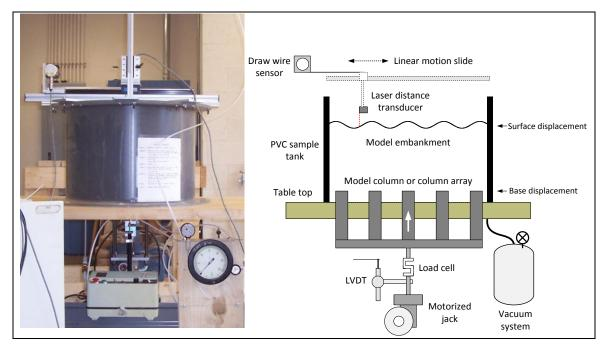
Figure 2: Photo and schematic of bench-scale test apparatus
