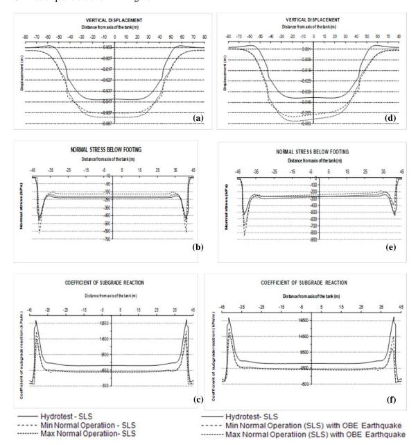
Figure 4: Settlement, normal stress and coefficient of subgrade reaction variations of the base slab for SLS cases at the end of Hydro-Testing, normal operation conditions with minimum pressures and maximum pressures without earthquake loading (a,b, c) and with OBE earthquake loading (d,e,f)
