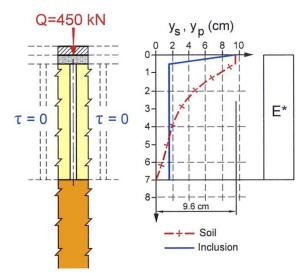
Figure 5: Step 1 of the calculation according to the simplified method - Cell mesh area 1,5  $m^2$ , vertical load case q = 200 kPa
