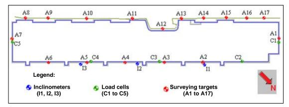
Figure 11: Location of the monitoring instruments.
