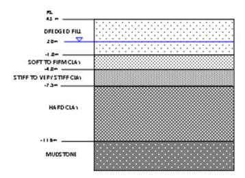
Figure 1 Simplified soil layering below the LNG tank
