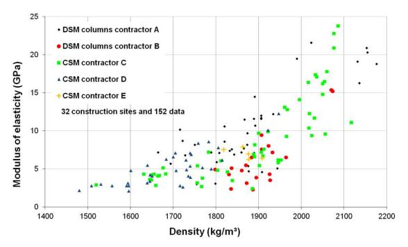
Figure 8: Relationship between the modulus of elasticity and the density of DSM material
