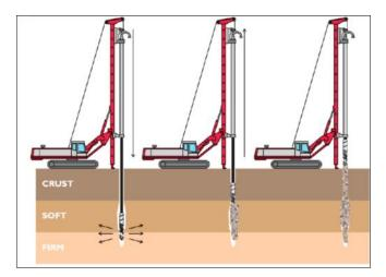
Figure 1: Typical CMC Installation Procedure
