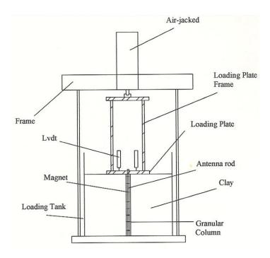
Figure 1: Sketch of the experiment setup
