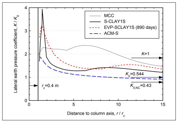
Figure 4: Change in lateral earth pressure for different soil models.
