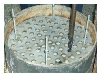
Photo 2: Clay is drilled with aid of prebored steel plate and auger
