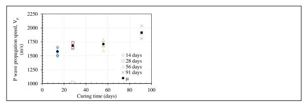
Figure 4: P wave propagation speed in soil-cement specimens with different curing duration
