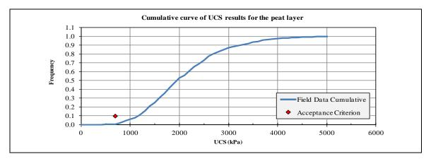
Figure 10: Statistical distribution of 28 days UCS for the peat layer (CF between 330 and 480 kg/m³)
