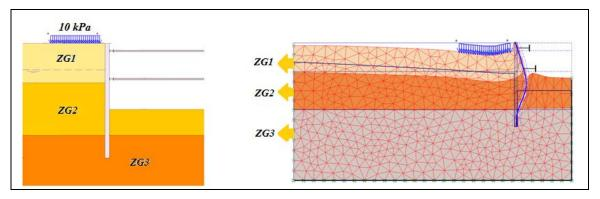
Figure 8: Section A: cross-section (on the left) and analysis model representing the deformation at the maximum excavation depth (on the right).
