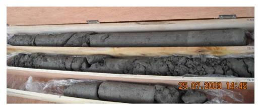
Figure 11: Cored Sample of a poorly constructed and non-uniform DSM column
