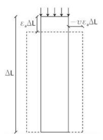
Figure 15: Illustration of the Poisson's ratio effect
