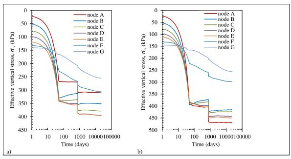
Figure 7: Vertical stress at output points in panel #2: a) SC1 case; b) SC2 case
