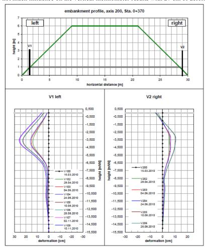
Figure 9: vertical inclinometer results at the 7 m high damm with drains and 600 kN/m geotextile
