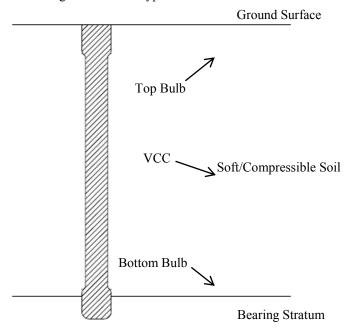
Figure 1: Typical VCC construction.
