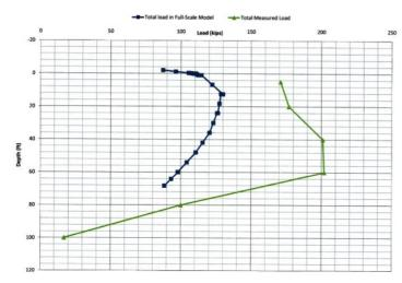
Figure 15: Load profile in CMCs - Actual vs. Model
