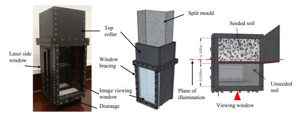
Figure 3: Experimental setup (a) test chamber (b) sample prepartion (after Ballacchino (2011))
