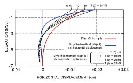
Figure 11: Comparison of the horizontal displacement profile calculated by Flac 3D model and the simplified method for a range of shear force boundary conditions T(0) at the inclusion head–Inclined load case  $q = 200 \text{ kPa } \theta = 10^{\circ}$
