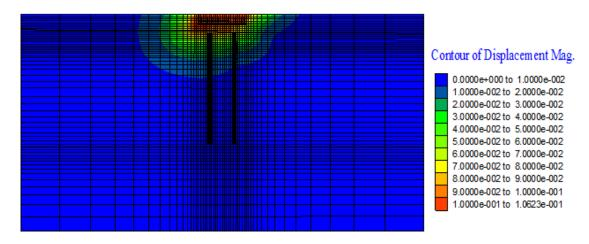
Figure 3: Displacement field - loading q=150 kPa inclined at  $\theta=20^{\circ}$
