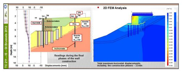
Figure 25: Horizontal displacements: measured and obtained through 2D FEM analysis.
