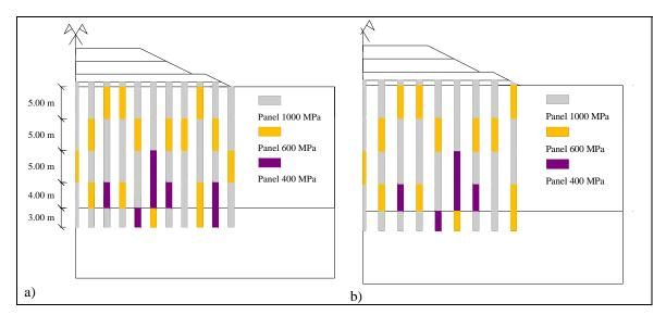
Figure 9: Models with weak zones in soil-cement panels: a) SC3 case; b) SC4 case
