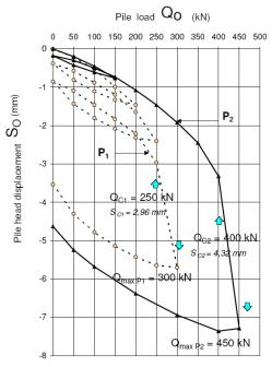
Figure 7: Load-settlement curve for column P1 and P2.
