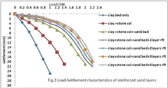
A loading intensity of 0.2 kN, as compared to unimproved sand bed, the settlement has been reduced by 15.3%, 43.2%, 57% respectively .For 0.6 kN, as compared to unimproved sand bed, the settlement has been reduced by 23%, 53.8%, 61.5% respectively. For 1.0KN the settlement has been reduced by 31%, 43%,47% respectively.
