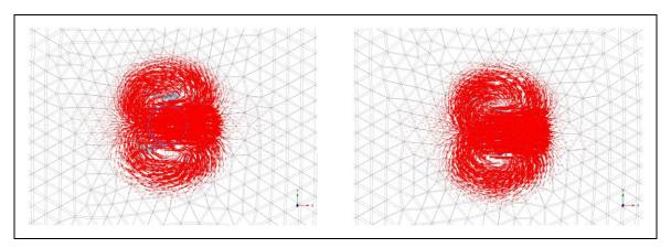
Figure 3: Displacement pattern around the pile at failure. Left: Volume pile; Right: Embedded pile
