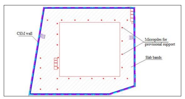
Figure 6: Plan view of the general configuration of the retaining wall structure.
