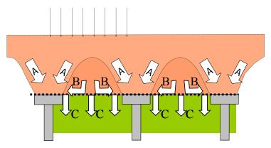
Figure 2: Load distribution in a piled embankment.
