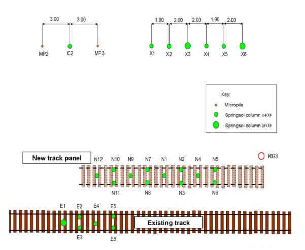
Figure 2: Location of soil-cement columns installed at Vernouillet.
