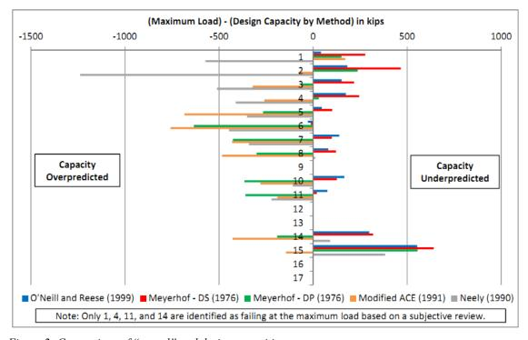
Figure 2: Comparison of "actual" and design capacities.
