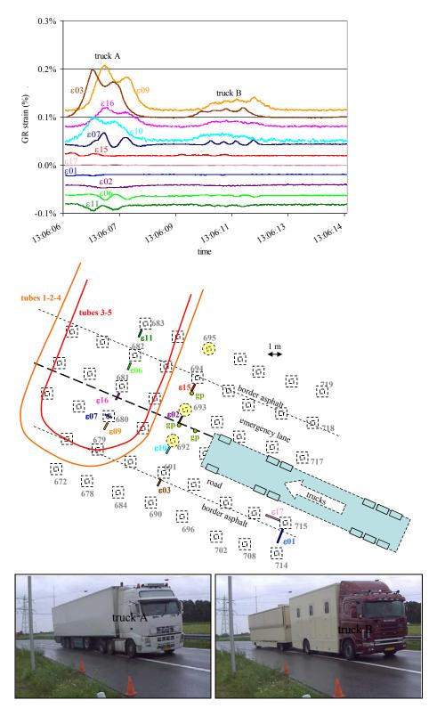
Figure 5: Measurements of the GR strains during the passage of two trucks on 6 September 2011.
