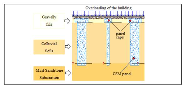
Figure 6: Cross-section of the performed solution.
