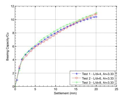
Figure 8: Load bearing characteristics of isolated stone columns
