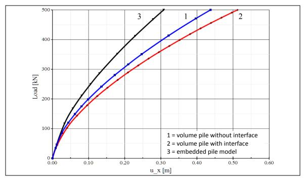
Figure 6: Load-displacement curves of pile top for different pile models
