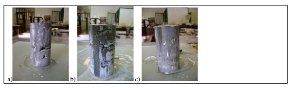
Photo 3: Soil-cements specimens prepared in laboratory: a) specimen # 28, rejected; b) specimen # 9, rejected; c) specimen # 26, tested under unconfined compression
