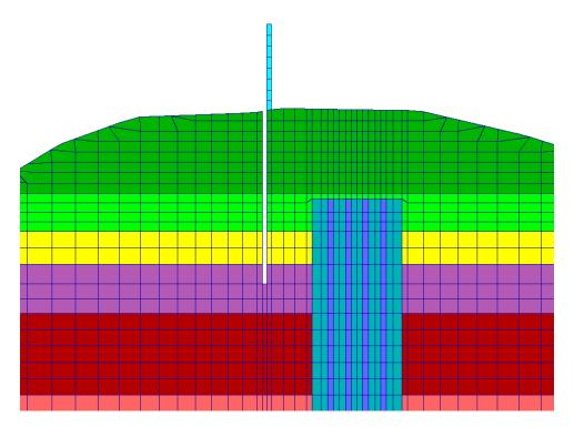
Figure 2: Consideration of water-filled gap in FLAC model
