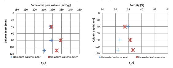
Figure 11: Cumulative pore volume and porosity distributions for the upper unloaded column (OR)
