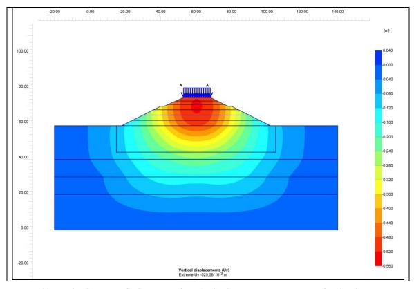
Figure 11: Total reduction in the forecast with PLAXIS HS cross section maximum dam height
