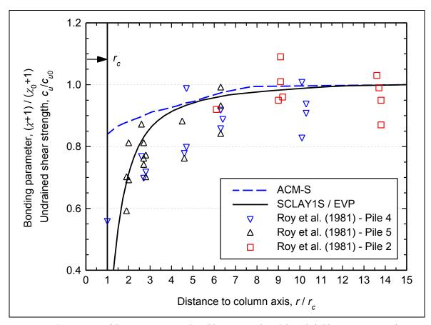
Figure 5: Comparison of destructuration predicted by numerical models with field measurements after undrained expansion of the cavity.
