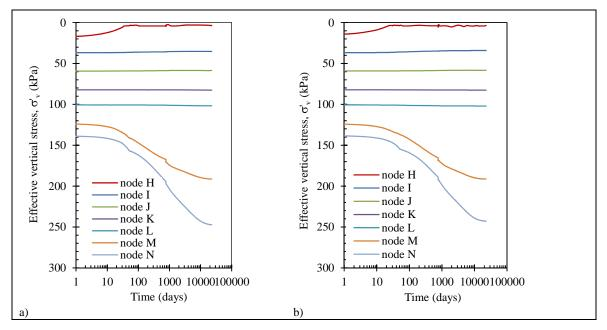
Figure 8: Vertical stress evolution at output points in soft soil: a) SC1 case; b) SC2 case
