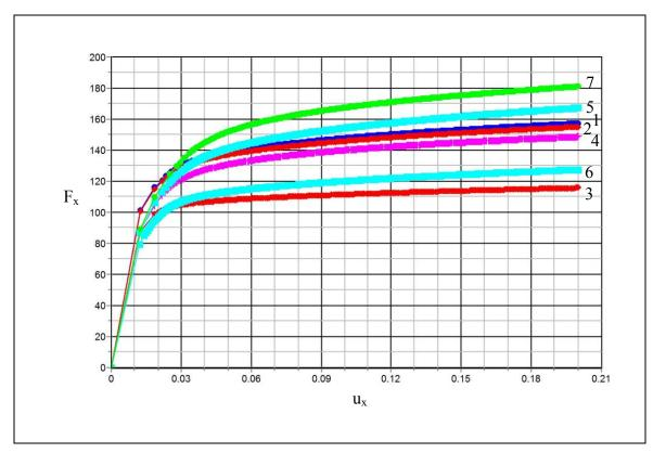
Figure 2: Load-displacement curves of different pile models – medium mesh density
