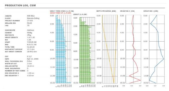
Figure 12: Typical production log (photo with courtesy of Malcolm Drilling Company)
