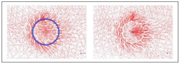
Figure 4:Major principal stresses around the pile at failure. Left: Volume pile; Right: Embedded pile
