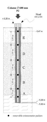
Figure 5: Removable extensometer in soil-cement
