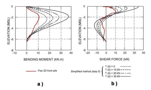
Figure 12: Comparison between Flac 3D results and simplified method results obtained with a range of shear force boundary conditions T(0) at inclusion head–Inclined load case q = 200 kPa  $\theta = 10^{\circ}$  (a) Bending moment (b) Shear force.
