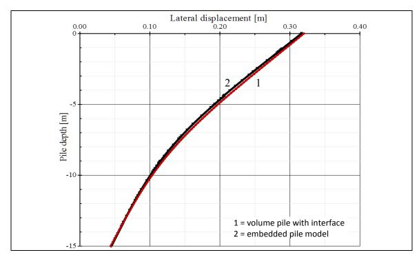
Figure 11: Pile deflection curves for different pile models
