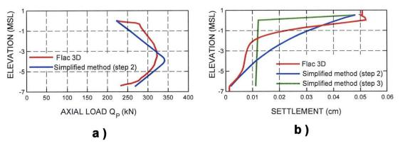
Figure 8: Comparison between simplified analytical method and numerical Flac 3D – Vertical load case q = 200 kPa. (a) Axial load in inclusions (b) Soil and pile settlement
