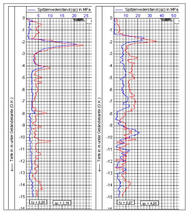
Figure 8: Pressure probe by comparison before and afterwards the vibro between the columns
