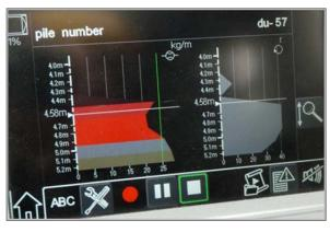
Photo11: PDE screen, visualisation of the column production
