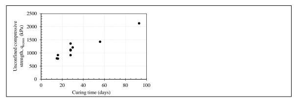
Figure 5: Evolution of maximum unconfined compression strength with curing time
