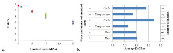
Figure 3: a. Variation of Young's modulus as a function of the percentage of unmixed material (surface area); b. Effect of the number of inclusions and their shape on the average Young's modulus for 30 numerical models (10% unmixed material)
