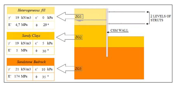
Figure 3: Main Geotechnical parameters and representation of a cross-section of the excavation.
