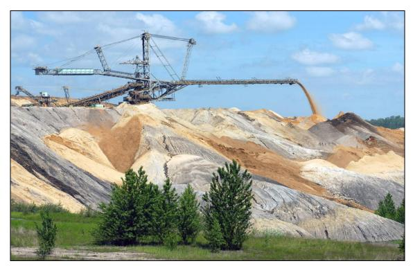
Photo 2: Development of the dump Schleenhain where the B176 is built on
