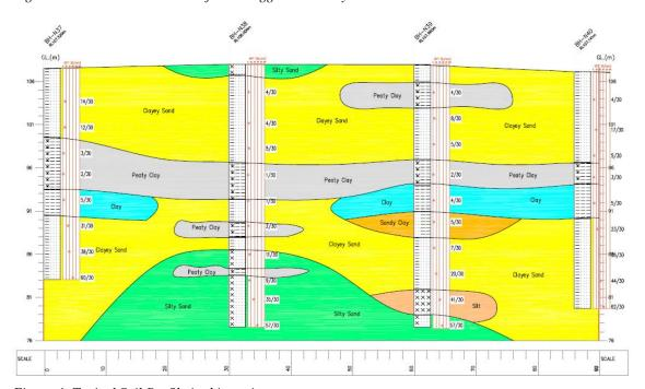
Figure 4: Typical Soil Profile in this project.
