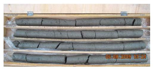
Figure 10: Cored Sample of a well-constructed and uniformly treated DSM column
