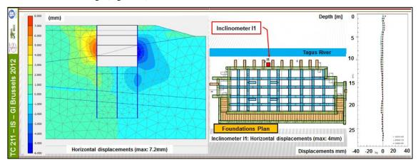
Figure 18: Main deformations obtained through FEM analysis and measured at the inclinometer 11.
