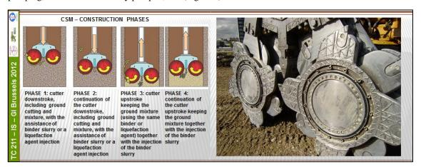
Figure 1: Main execution sequence of the CSM technology and view of the cutter wheels.
