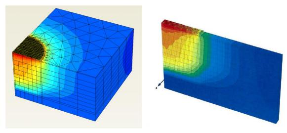
Figure 5: Results of 3D FEM analysis for quarter of tank model (left) and thin slice model (right)
