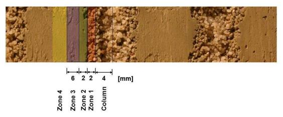
Figure 1: Spatial distribution of the installation effects around stone columns (Weber, 2008)
