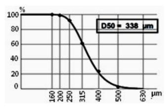
Figure 1: Particle size distribution curve for Hostun sand
