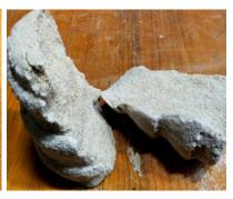
Figures 6a-6b-6c: on the left, unloaded column and damaged column from test 2 - in the middle, failure of SM specimen taken from test 2 after a UCS test- On the right, failure of SM specimen taken from test 3 after a UCS test.
