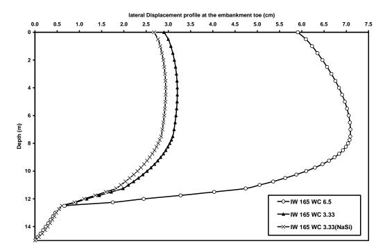
Figure 5: Horizontal Displacement profile at the toe of the embankment supported on DMCC columns
