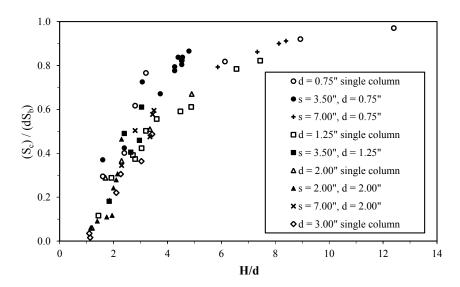
Figure 10: Measurements of the ratio of surface settlement over the column axis to maximum differential base settlement versus sample height divided by column diameter for unreinforced bench-scale tests performed using dry sand prepared at Dr = 87%.
