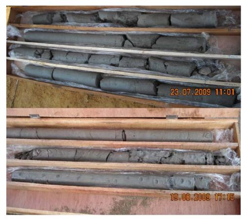
Figure 8: Coring Samples Photo showing some inconsistent results
