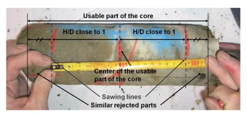
Figure 8: Preparation of two DSM test specimens, both intended for UCS tests
