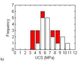
Figure 19: Distribution of the UCS values from 2 different sites. The samples with inclusions larger than 1/6 of the specimen diameter are indicated in red: a) 6 on a total of 51 samples; b) 9 on a total of 26 samples
