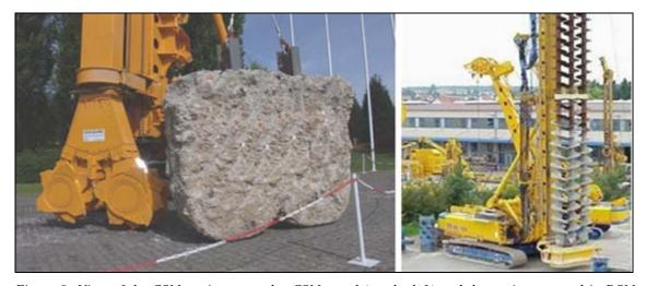
Figure 9: View of the CSM equipment and a CSM panel (on the left) and the equipment used in DSM technology (on the right).
