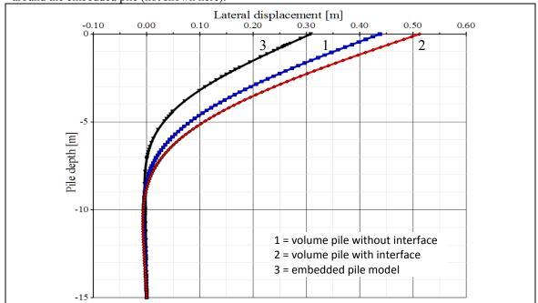
Figure 7: Pile deflection curve for different pile models
