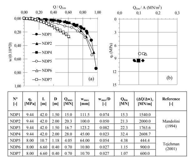
Figure 2: Experimental data for NDP: (a) non-dimensional curves; bearing capacity indicator (b).
