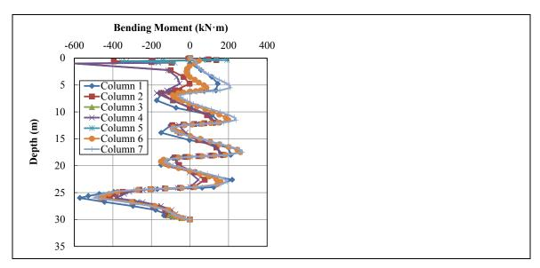
Figure 8: Bending moment diagram of the seven rows of drilled shafts (columns) for Case 21
