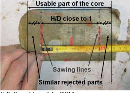
c) Drawing of the second sawing line
