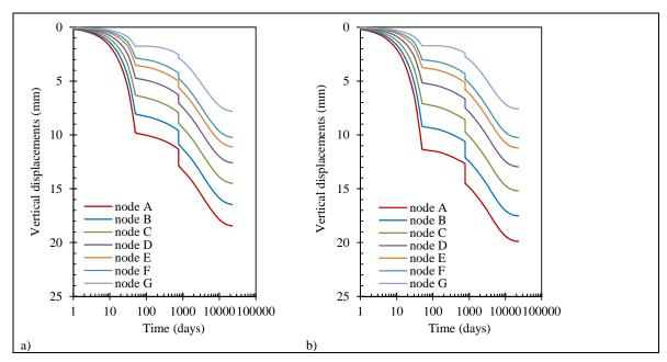
Figure 4: Time history of settlements at output points; a) panel #2, SC1 case; b) panel #2, SC2 case
