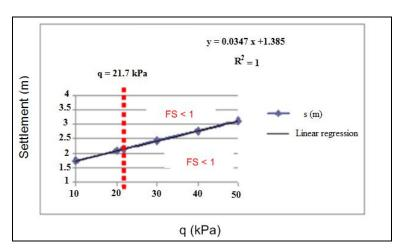
Figure 3: Settlement prediction vs load intensity by Columns software
