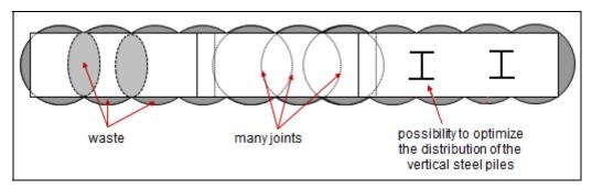
Figure 10: Comparison between rectangular soil-cement panels (CSM technology) and circular soil-cement columns (DSM technology).
