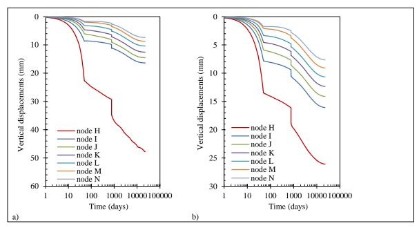
Figure 5: Time history of settlements at output points: a) soft soil, SC1 case; b) soft soil, SC2 case
