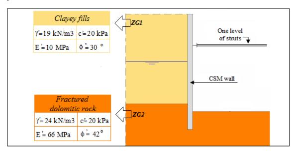
Figure 3: Main geotechnical parameters and cross-section of the excavation.
