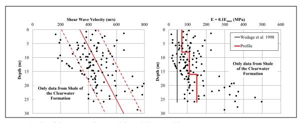
Figure 2: Plot of shear wave velocity and derived elastic modulus
