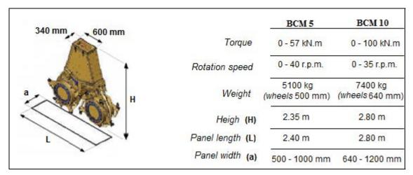
Figure 3: Characteristics of the Cutter Heads BCM 5 and BCM 10 (Bauer Maschinen).
