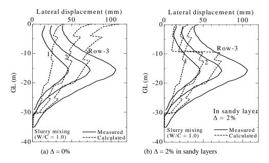
Figure 6: Comparison of measured and calculated lateral displacement profiles at site-1
