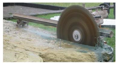
Figure 4: Sawing of a CSM panel
