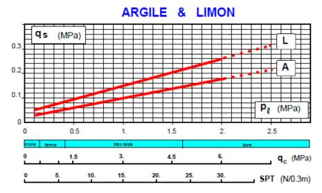
Figure 12: Abacus for the calculation of shaft friction qs in jet grouting columns for silt and clay [3]
