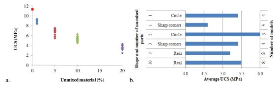
Figure 4: a. Variation of UCS values as a function of the percentage of unmixed material (surface area); b. Effect of the number of inclusions and their shape on the average UCS value for 30 numerical models (10% unmixed material)
