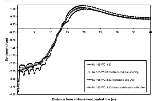
Figure 7: Vertical Displacement profile along base of the embankment supported on DMCC columns
