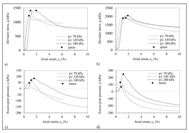
Figure 7: Stress-strain response in confined triaxial compression: a) q- $\varepsilon_a$  plot for 31/32 curing days; b) q- $\varepsilon_a$  plot for 92/93 curing days; c) u- $\varepsilon_a$  plot for 31/32 curing days; d) u- $\varepsilon_a$  plot for 92/93 curing days
