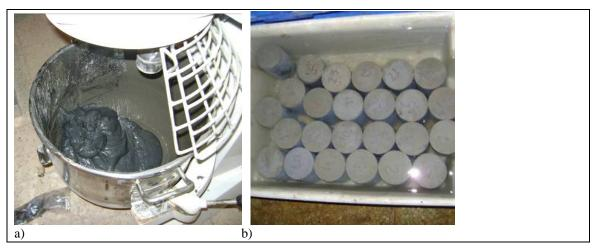
Photo 2: Preparation of soil-cement specimens: a) soil (dark) mixed with the cement slurry; b) soil-cement specimens in a container with water from the Jardim do Tabaco dock
