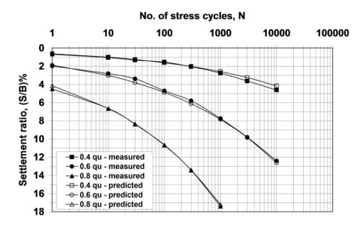
Figure 2: Number of stress cycles & settlement ratio of untreated soil
