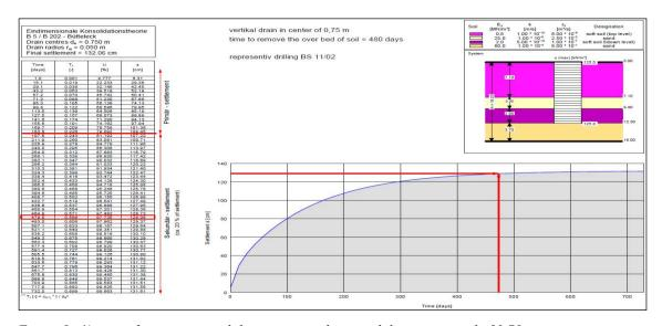
Figure 5: ½ year of primary consolidation even with vertical drains in a grid of 0.75 m
