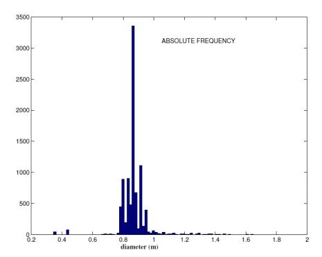
Figure 3: Histogram of the diameter of stone columns. Dry method (bottom feed)
