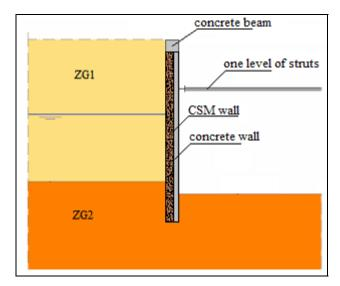
Figure 7: Cross-section of the retaining wall.
