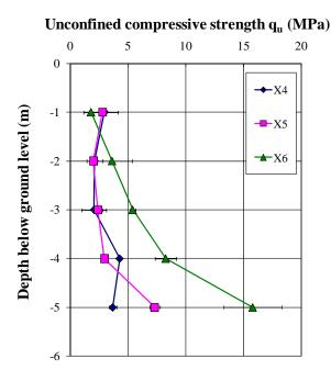
Figure 3: Unconfined compressive strength  $q_u$  versus depth for columns X4, X5 and X6.
