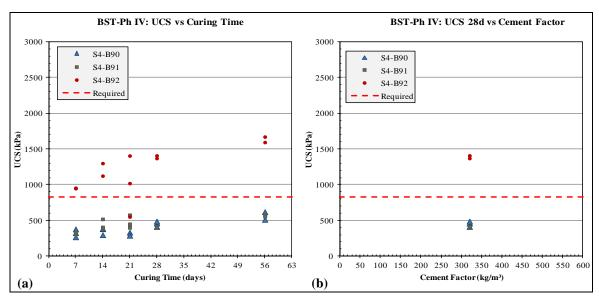
Figure 7: BST - Phase IV results (a) UCS vs Curing time; (b) 28 days UCS vs Binder Factor
