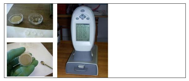
Photo 5: Preparation of the XRF samples for cement content determination, with the equipment NITON series XLI 700 Analyser (Jorge et al., 2009)
