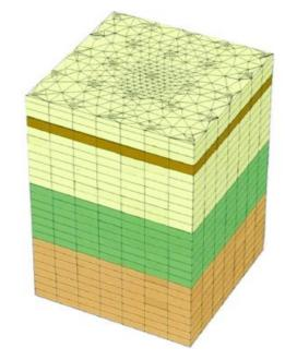
Figure 3: Example of 3D FEM model for support of slab and footings on CMCs
