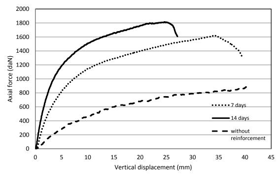
Figure 5: Evolution of the bearing capacity of foundation in terms of vertical displacement.
