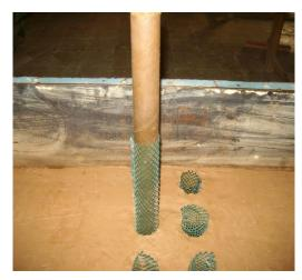
Photo1: Construction of encased stone columns
