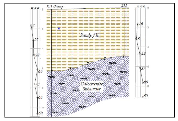
Figure 6: Geological-geotechnical profile (S11 and S12).
