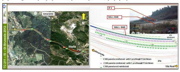
Figure 21: Location and plan of the walls.
