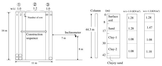
Figure 7: Plan view of the layout of columns and construction sequence
