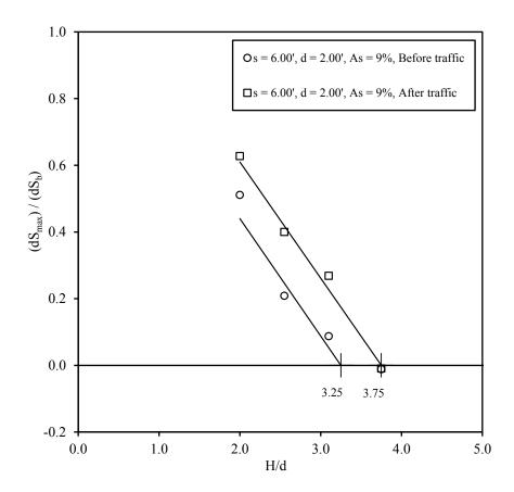
Figure 8: Ratio of maximum differential surface settlement to maximum differential base settlement versus sample height divided by column diameter. Labels indicate  $H_{crit}/d$  evaluated before and after trafficking.
