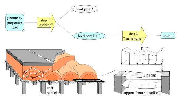
Figure 1: The calculation of the GR strain due to vertical load is carried out in two steps.
