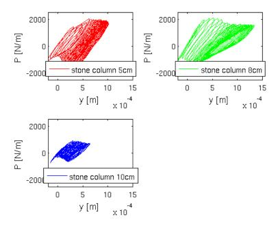
Figure 8: p-y curves obtained at pile head for experiments with 5cm, 8cm and 10 high stone column
