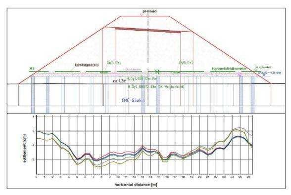
Figure 10: horizontal inclinometer results with arround  $1\ cm$  of CMC settlements and  $2\ cm$  of reinforced earth settlements
