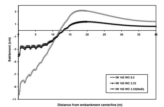
Figure 4: Vertical Displacement along base of the embankment supported on DMC columns
