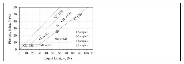
Figure 2: In situ soil samples position in plasticity chart
