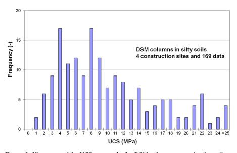
Figure 3: Histogram of the UCS test results for DSM column systems in silty soils
