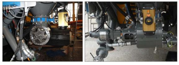
Photo 1: Star feeder with butterfly valve and silo; Photo 2: Rotary valve with hydraulic motor, gear box and coupling
