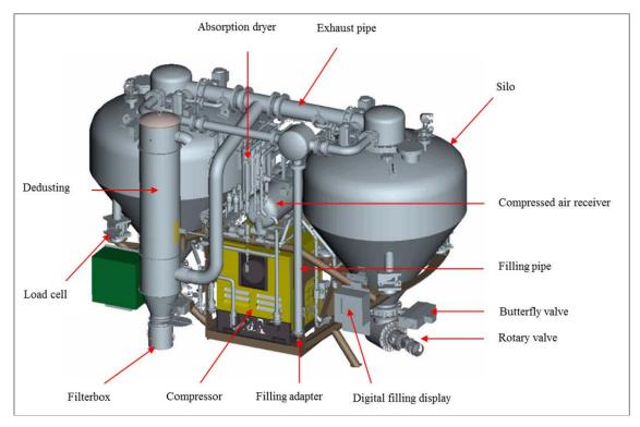
Figure 4: Lime cement station [Liebherr – BVV 2010]
