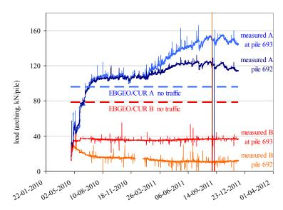
Figure 4: Results of field measurements near Woerden, see also Figure 5. Subgrade reaction k in predictions: k = 0 kN/m3 (no subsoil).
