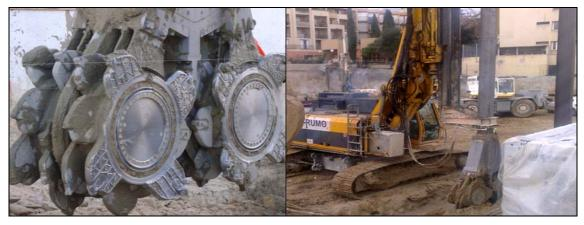
Figure 3: Detail of the cutting wheels (on the left) and general aspect of the hidromill (on the right).
