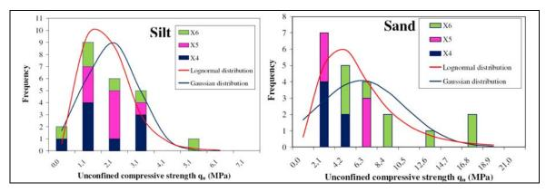
Figure 4: Histograms of  $q_u$  obtained on cored samples from columns X4, X5 and X6.
