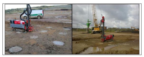
Photo 6: Execution of the Ménard pressuremeter
