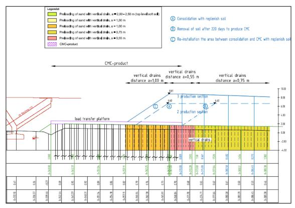
Figure 3: steps of consolidation and construction
