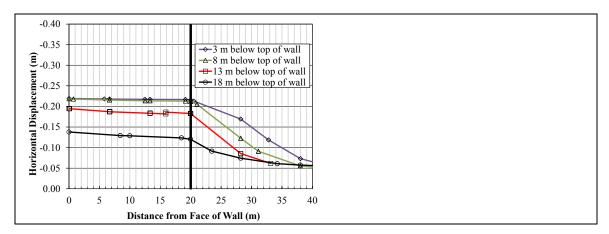
Figure 7: Plot of horizontal displacement of the soil adjacent to the reinforcement as a function of the distance from the face of the wall
