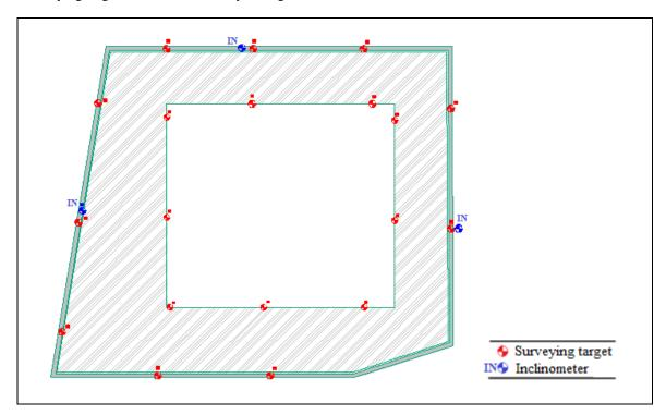
Figure 13: Surveying targets and inclinometers installed according to the monitoring plan of the work.
