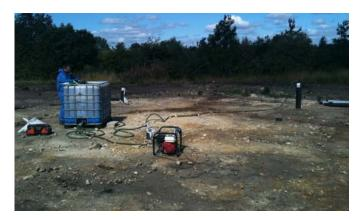
Figure 9: Pumping from one of the PRB walls.
