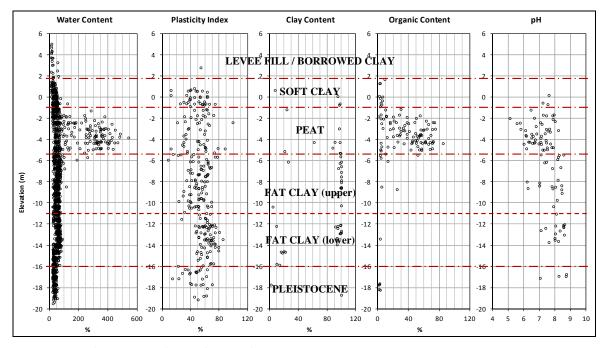
Figure 3: Soil properties plots and interpolation
