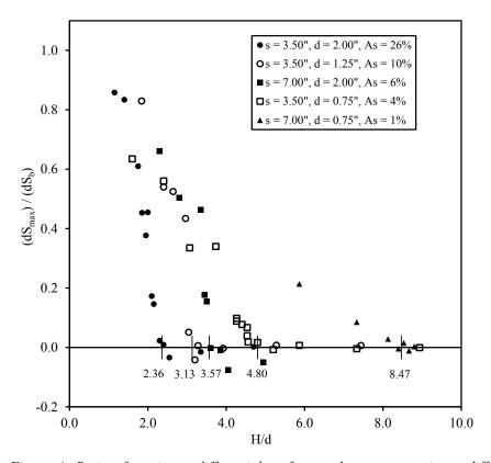
Figure 4: Ratio of maximum differential surface settlement to maximum differential base settlement versus sample height divided by column diameter for samples without reinforcement prepared dry at  $D_r = 87\%$ . Labels indicate  $H_{crit}/d$  for each of the unit cell geometries evaluated.
