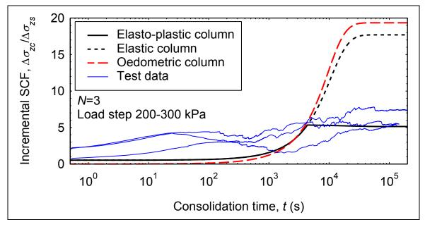
Figure 4: Incremental stress concentration factor (SCF) with time.
