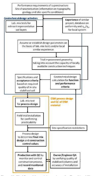
Figure 10: Workflow of deep-mixing project, after Terashi and Kitazume (2011)
