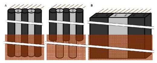
Figure 2: Schematic plan view of the secant execution of (A) cylindrical DSM columns and (B) rectangular DSM panels
