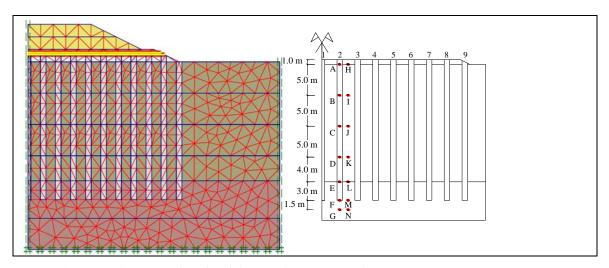
Figure 2: Finite element mesh and nodal points for output results representation
