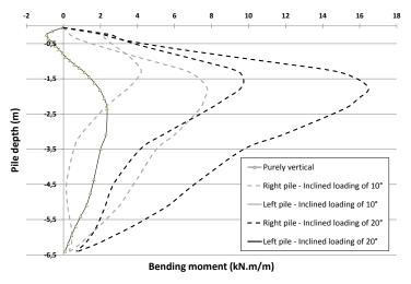
Figure 4: Bending moment for different load inclinations - q=150kPa
