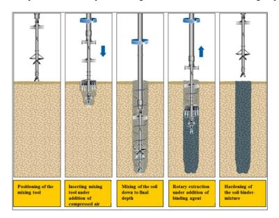
Figure 1: Schematic production steps [Liebherr - BVV 2010];
