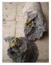
Figure 13: Photos of soil-cement samples before and after UCS tests
