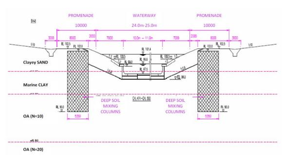
Figure 6: Typical Scheme of DSM for enhancing the slope stability of Punggol Waterway
