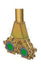
Figure 4: CSM Cutter Head
