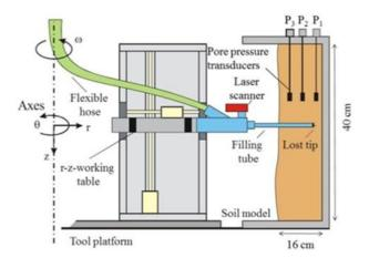
Figure 7: Stone column installation tool (Weber, 2008)
