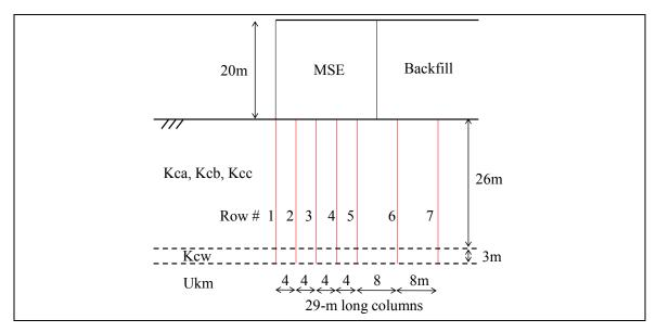
Figure 3: Schematic cross section layout of Geometry 4
