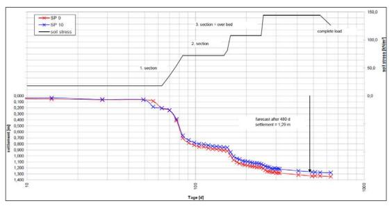
Figure 8: measurment at the settlement plates SP 9 und SP10.
