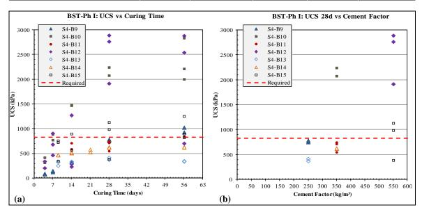
Figure 4: BST - Phase I results (a) UCS vs Curing time; (b) 28 days UCS vs Binder Factor
