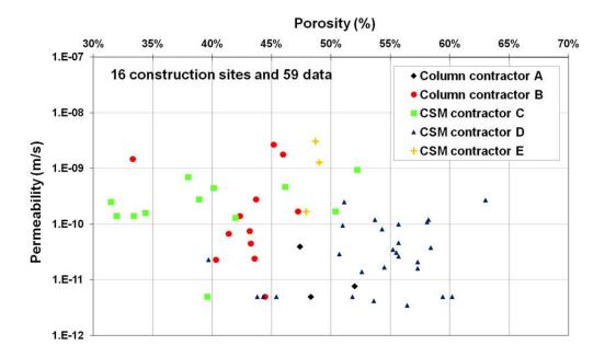
Figure 14: Relationship between permeability and porosity for DSM cores
