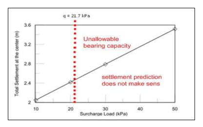
Figure 2: Consolidation settlement versus load intensity (Plaxis) at centre line of embankment [4]
