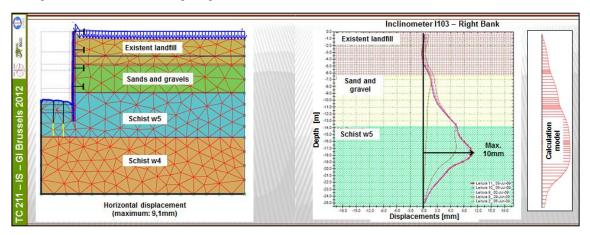
Figure 7: View of the adopted FEM model and horizontal displacements.
