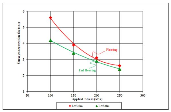
Figure 7: Variation of n value with applied surface pressure
