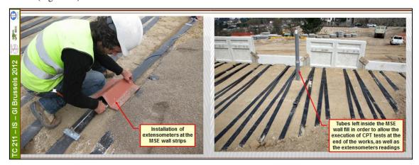
Figure 30: Devices adopted for monitoring the "Marão" Motorway M4B wall.
