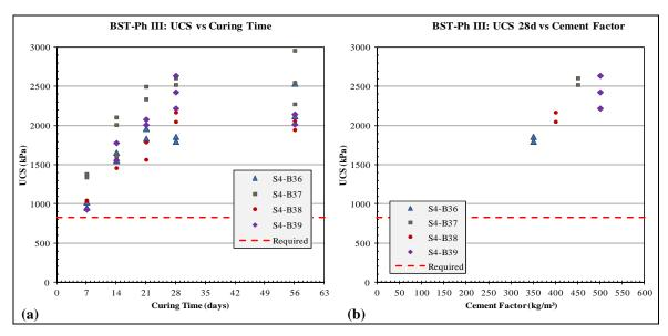
Figure 6: BST - Phase III results (a) UCS vs Curing time; (b) 28 days UCS vs Binder Factor
