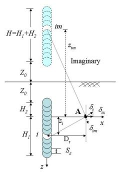
Figure 2: Vertical section illustrating the lateral displacement in the x direction caused by installation of a single soil-cement column (after Chai et al. 2009)
