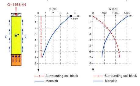
Figure 6: Step 2 of the calculation according to the simplified method - Monolith cross-section area  $2.8 \text{ m}^2$ , vertical load case q = 200 kPa
