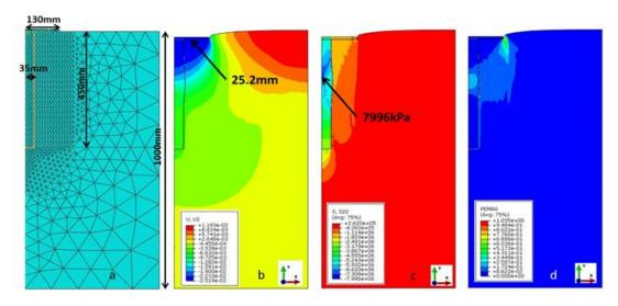
Figure 8: Numerical modeling results for reinforced soil (14 days after column installation): a- mesh and model dimensions, b- map of vertical displacement  $U_v$ , c- map of axial stress  $\sigma_{vv}$ , D) plastic zones
