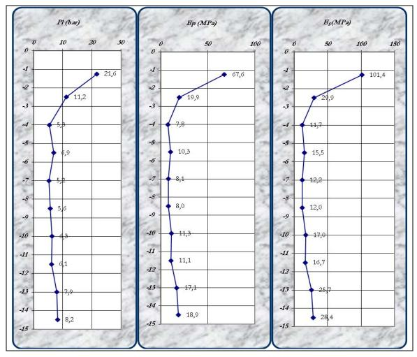
Figure 3: Pressuremeter test results of section 15, before soil improvement with representation boundary pressure Pl, Ménard modulus Ep and stiffness modulus Es on the depth
