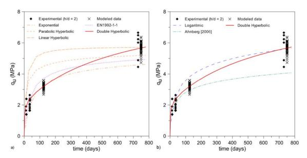
Figure 7: influence of curing time on strength development for treated clayey soil from Bologna: a) comparison between double hyperbolic formulation and classical models proposed for concrete; b) comparison between double hyperbolic formulation and some proposed for DMM.
