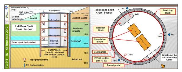
Figure 6: Cross section and plan of the adopted solutions.
