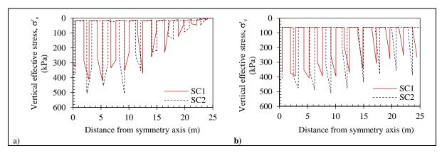
Figure 6: Vertical effective stress after calculation phase #6 completion: a) embankment base; b) at depth 10 m
