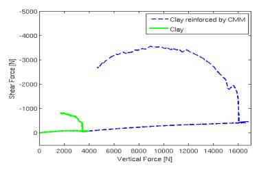
Figure 3: Swipe test for clay and soil reinforced by CMM®
