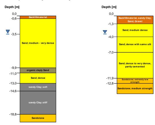
Figure 3: Example borehole logs; left for socketing into clay (2 m); right socketing into Sandstone (1 m)
