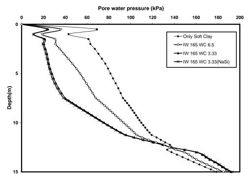
Figure 6: Pore Pressures distribution beneath center of embankment
