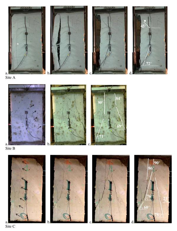
Photo 1: Pictures taken from the loaded block from the three sites, illustrating the occurrence of fractures during loading
