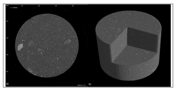
Figure 4: micro-CT analysis of a CSM treated speciment: a) 2D cross section; b) 3D reconstruction.
