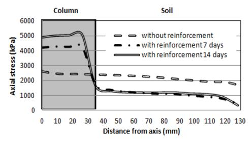
Figure 9: Axial stress distribution under foundation
