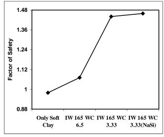
Figure 3: Influence of column properties on Factor of Safety
