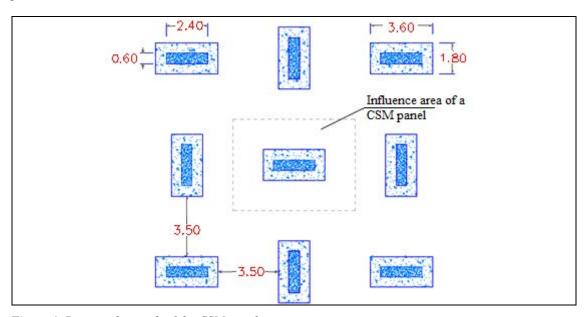
Figure 4: Rectangular mesh of the CSM panels.
