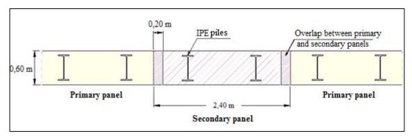
Figure 4: Representation of the overlapping of primary and secondary panels of the CSM retaining wall.
