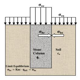
Figure 1: Distribution of stresses in the unit cell
