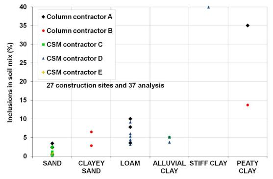
Figure 18: Percentage of soil inclusions in DSM material
