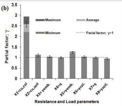
Figure 5: a) Design values and b) partial factors evaluated from RBD analysis for the resistance and the load parameters. The resistance parameters rank is varying from (X1 to X4), while the load parameters rank is varying from (X5, X8)
