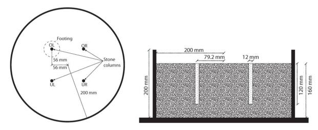
Figure 5: Layout of the stone columns
