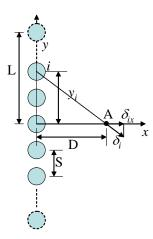
Figure 1: Plan section illustrating the lateral displacement in the x direction caused by installation of a single row of soil-cement columns (after Chai et al. 2005)
