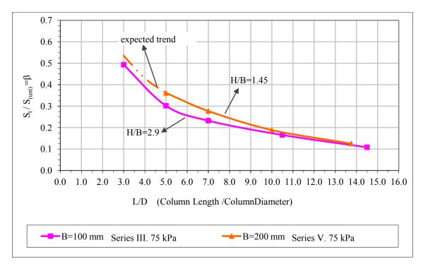
Figure 3:  $\beta$  – L/D relation for series III and V for 75 kPa loading
