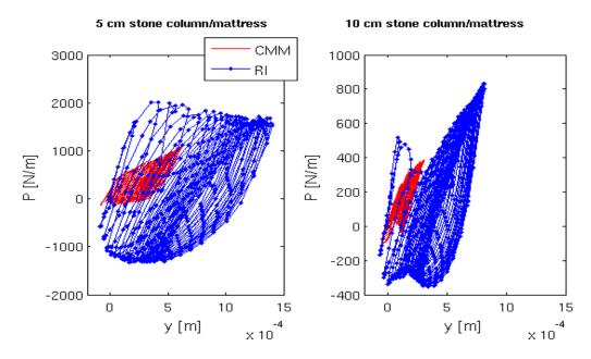
Figure 9: P-Y loops at the top of the rigid inclusion for the two soil improvement technologies
