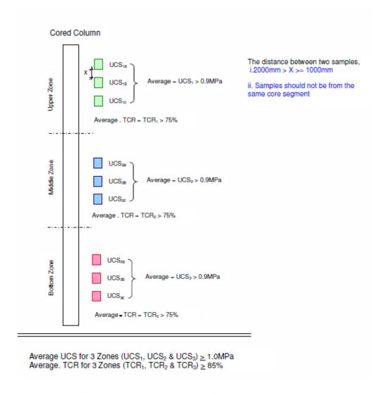
Figure 9: Revised Acceptance Criteria for DSM Column
