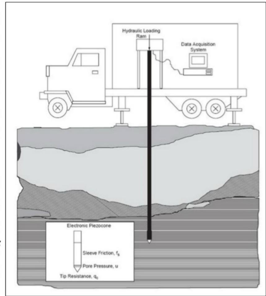
Figure 2.0 : Cone Penetration Test
