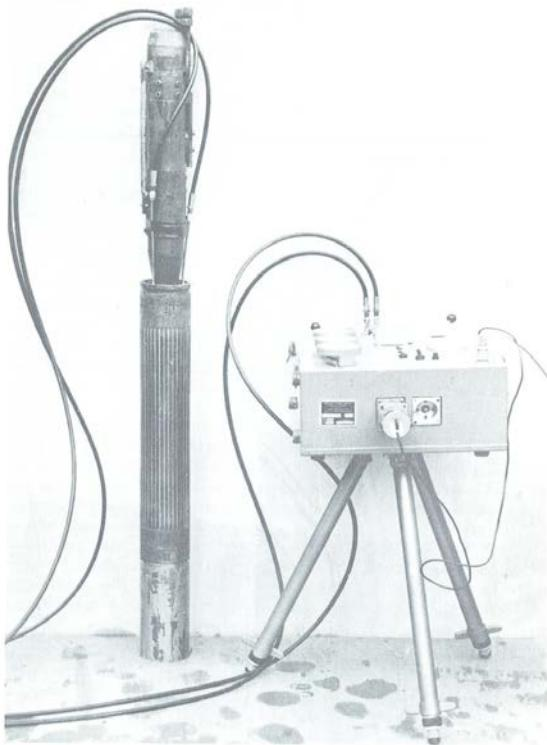
Fig. 6-39: Probe and control unit for a self-boring pressuremeter for hard soil (PAFSOR or PAF-72).
