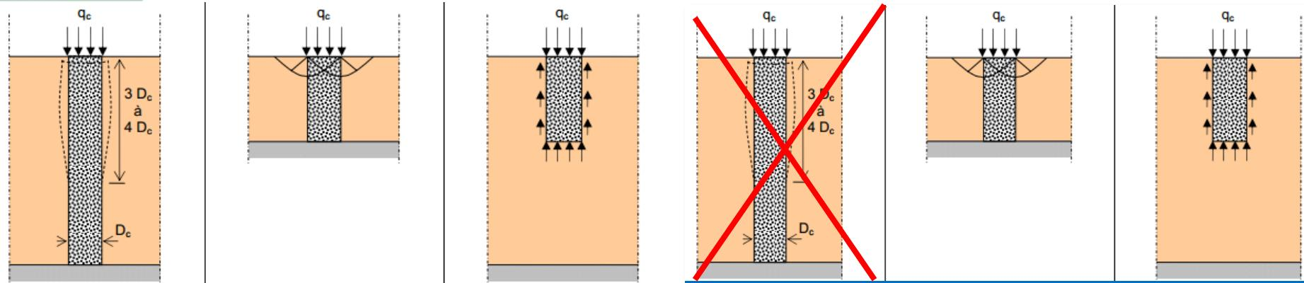
Failure by Lateral Expansion ( bulging )
