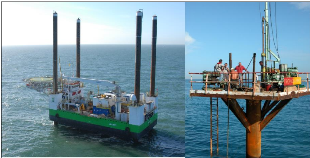
Figure 8: Stable working platforms for nearshore marine site investigations: jack-up platform Vagant (left) and monopole (right)
