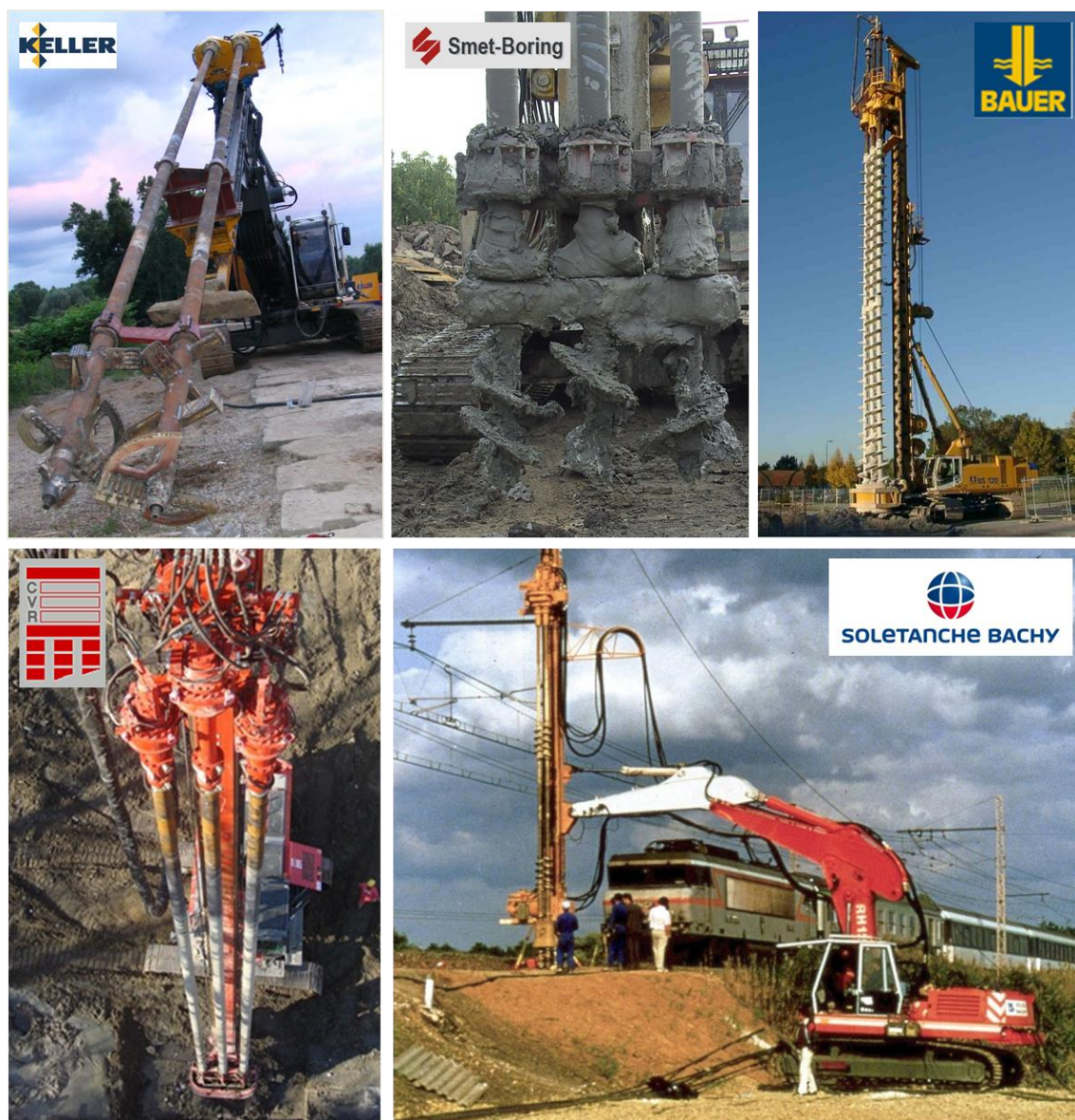
Figure 10: Wet mixing systems in double and triple shaft configurations, after Topolnicki (2012), Denies (2012) and Borel (2012) with the courtesy of Keller, Smet-Boring nv, Bauer, CVR nv and Soletanche Bachy
