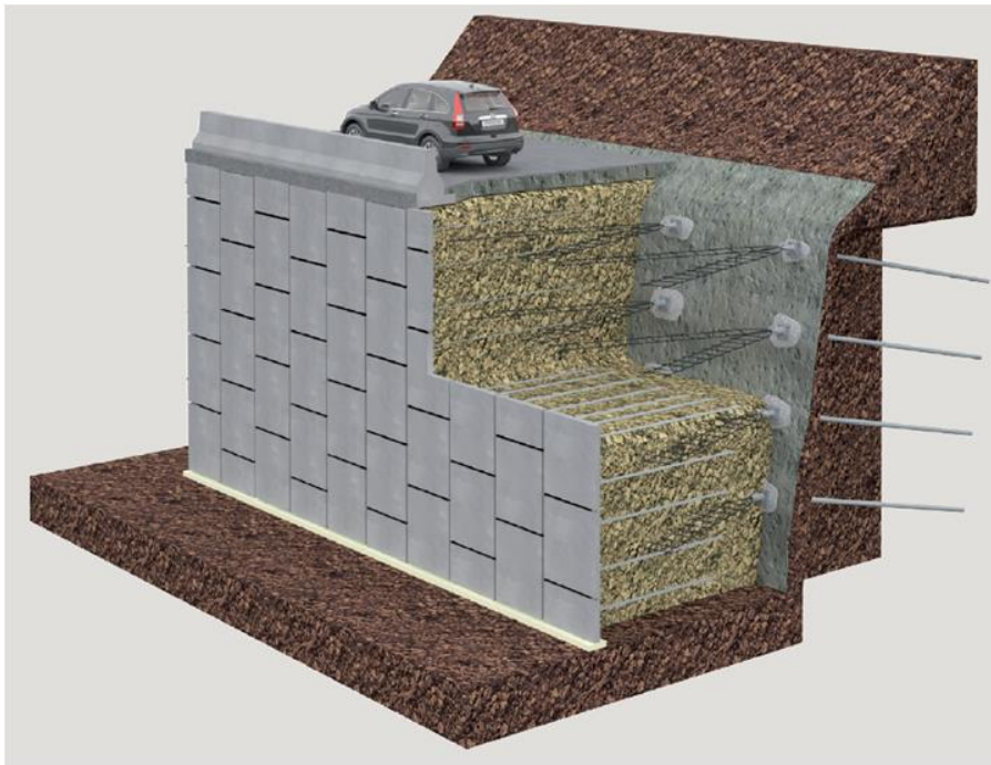
Figure 41: Combination of MSE-wall with soil nailing
