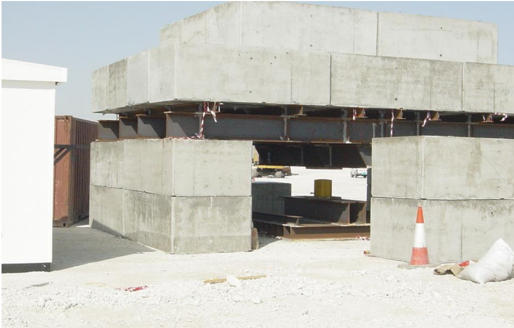
Figure 59: Typical zone load test set-up
