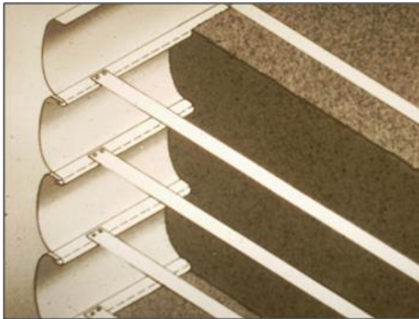
Figure 28: Concept of original Terre Armée
