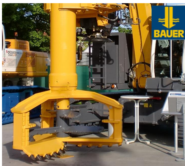
Figure 7: Bauer Single Column Mixing-Double Head, SCM-DH system (available tool diameter for single shaft ranging between 180 and 240 cm), after Topolnicki (2012) with the courtesy of Bauer
