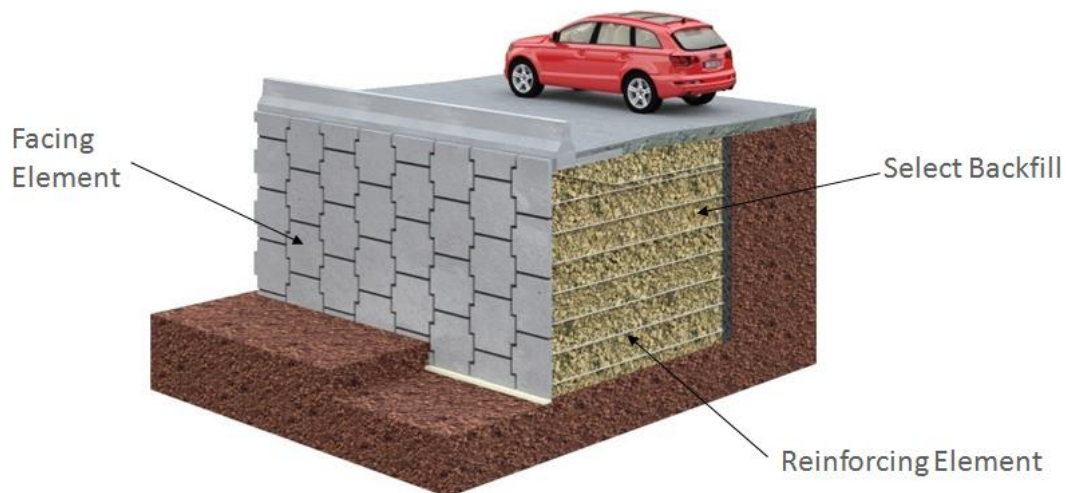
Figure 29: Basic components of an MSE-wall
