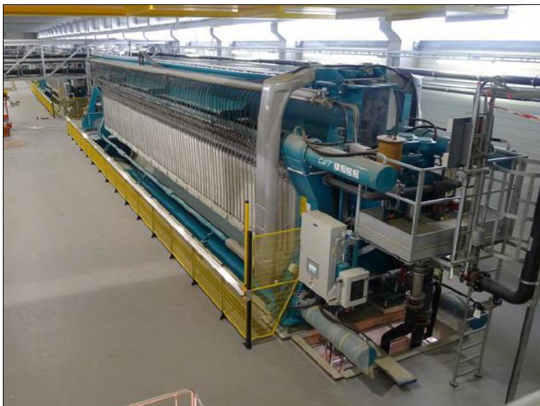
Figure 53: Mechanical dewatering by chamber filter presses at the Amoras project, Antwerp, Belgium
