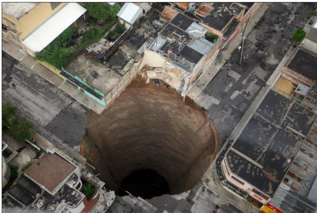
Figure 5: 18 m diameter sinkhole in Guatemala City (2010)
