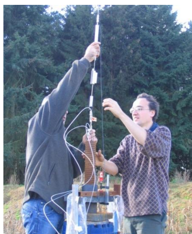
Figure 65: Installation of a retrievable instrumentation system in a reservation tube installed in a vertical anchor, from Huybrechts (2012)
