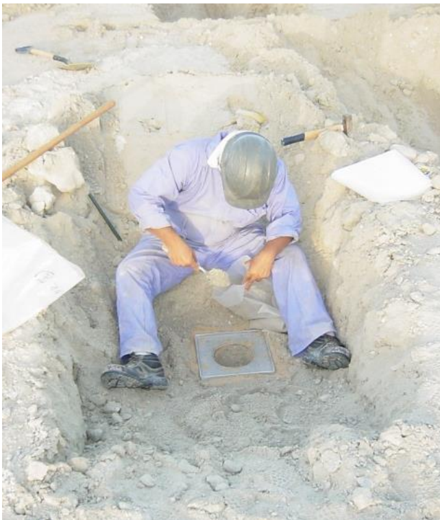
Figure 58: Technician performing in-situ density determination at 1 m deep excavation by applying the sand replacement method
