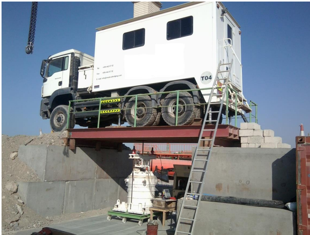
Figure 61: Typical set-up for onsite calibration chamber testing
