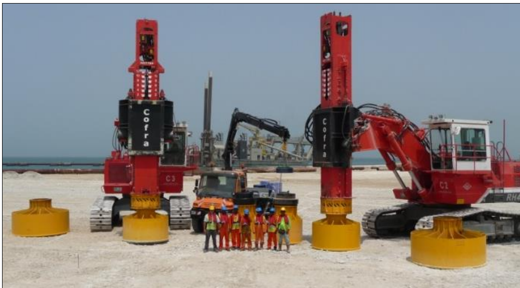
Figure 19: Rapid Impact Compaction equipment (Cofra Group)
