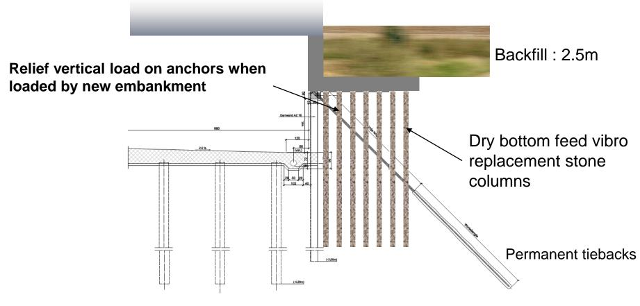
Tiebacks between rows of columns (unbonded length)
